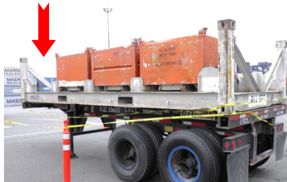
Photo 4: Cone bins set on flat racks loaded on to an intermodal chassis trailer. The arrow indicates the location of the bin that the victim had lifted and elevated on the forks of the forklift.
