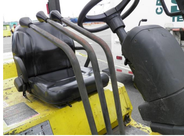
Photo 9: Forklift control levers used to adjust the forks and mast. The middle lever is the mast tilt lever.
