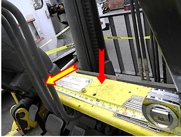
Photo 8: Forklift dash (red arrow) upon which the victim was standing when his foot inadvertently pushed against the mast tilt lever (yellow arrow). View is from inside the operator's cab.
