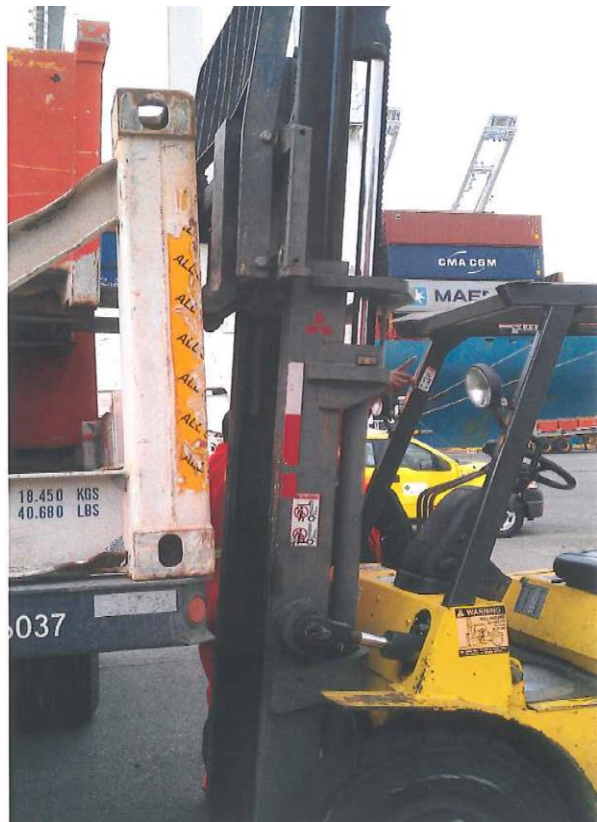
Photo 7: Recreation of the position of the forklift just before the incident. The forklift is next to the intermodal chassis trailer with a bin elevated on its forks. The victim climbed on to the forklift's dashboard between the mast and overhead guard to look into the bins on the trailer.
