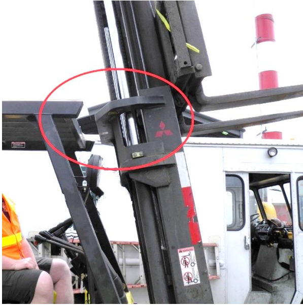
Photo 5: Forklift mast in the full tilted back position. The red circle indicates the area where the victim's torso was crushed between the cross member of the overhead guard and the mast.
