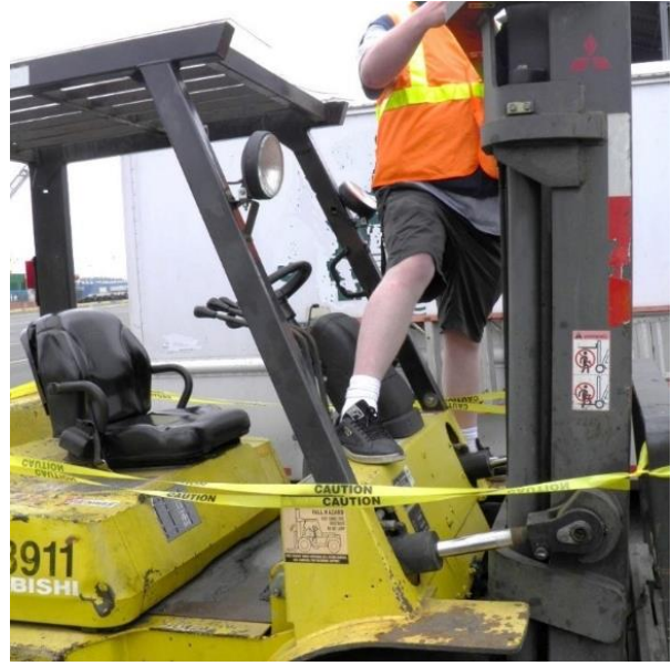
Photo 6: A longshore worker demonstrates how the victim might have accessed the forklift's dash to look into the bin elevated on the forklift's forks. The victim was standing with both feet on the dash when his right foot inadvertently activated the forklift control on the dash that caused the mast to tilt backwards, crushing him against the operator's cab overhead guard.
