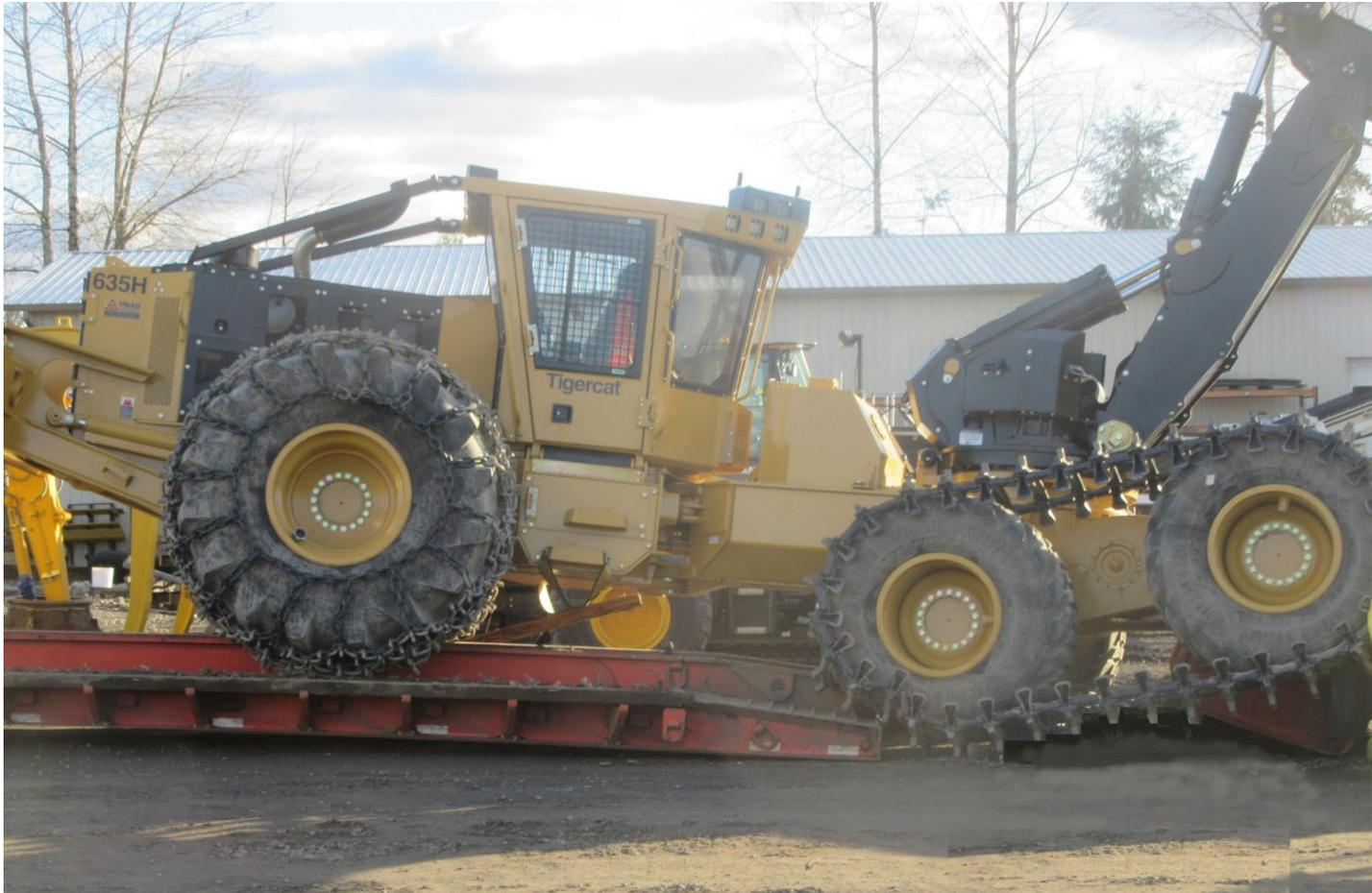
**Photo 3.** Skidder with tracked bogie wheels between lowboy trailer's lowered flatbed deck and detached gooseneck.
