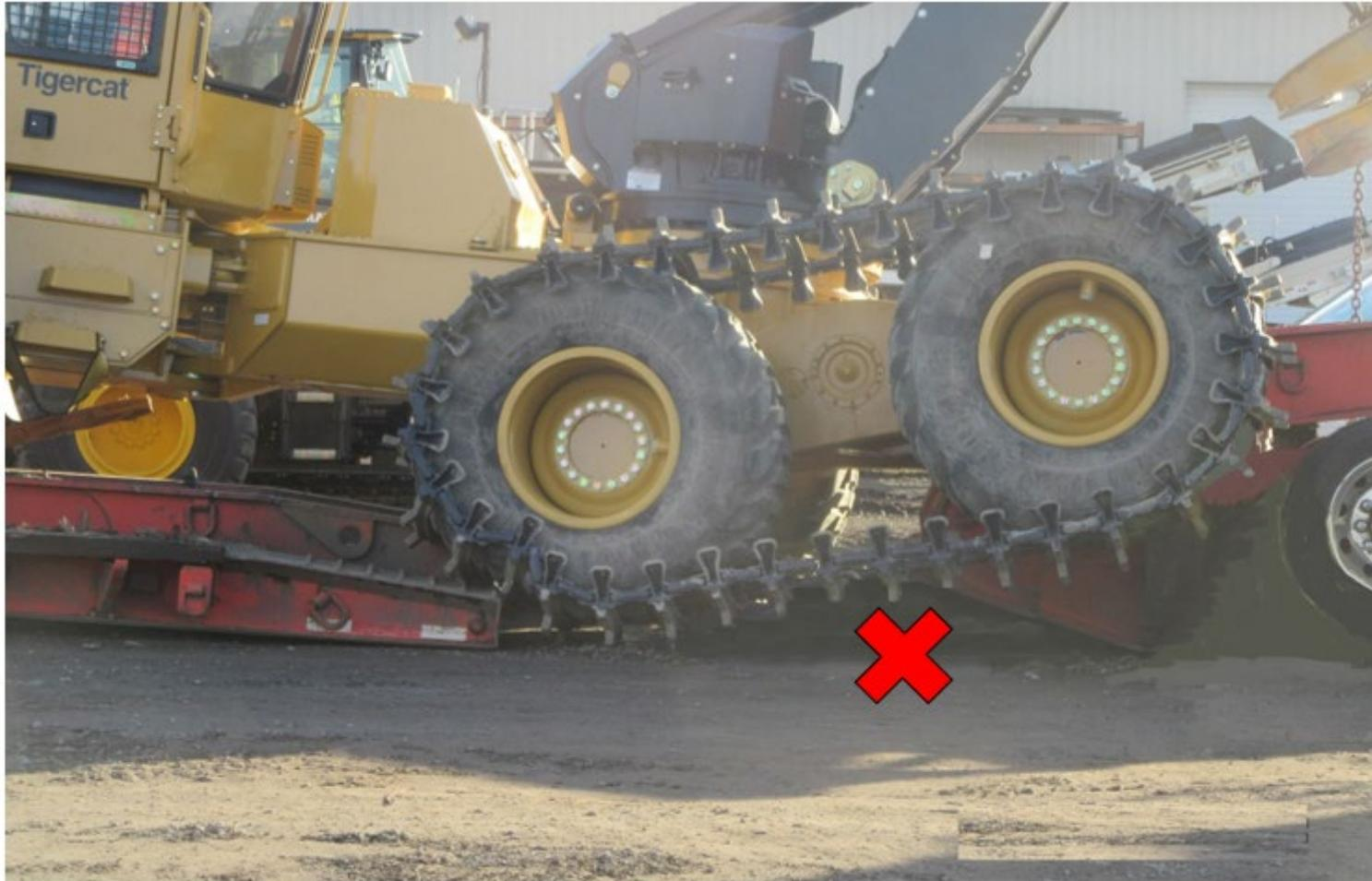
**Photo 2.** The owner was crushed under the skidder's tracked bogie wheels (X).
