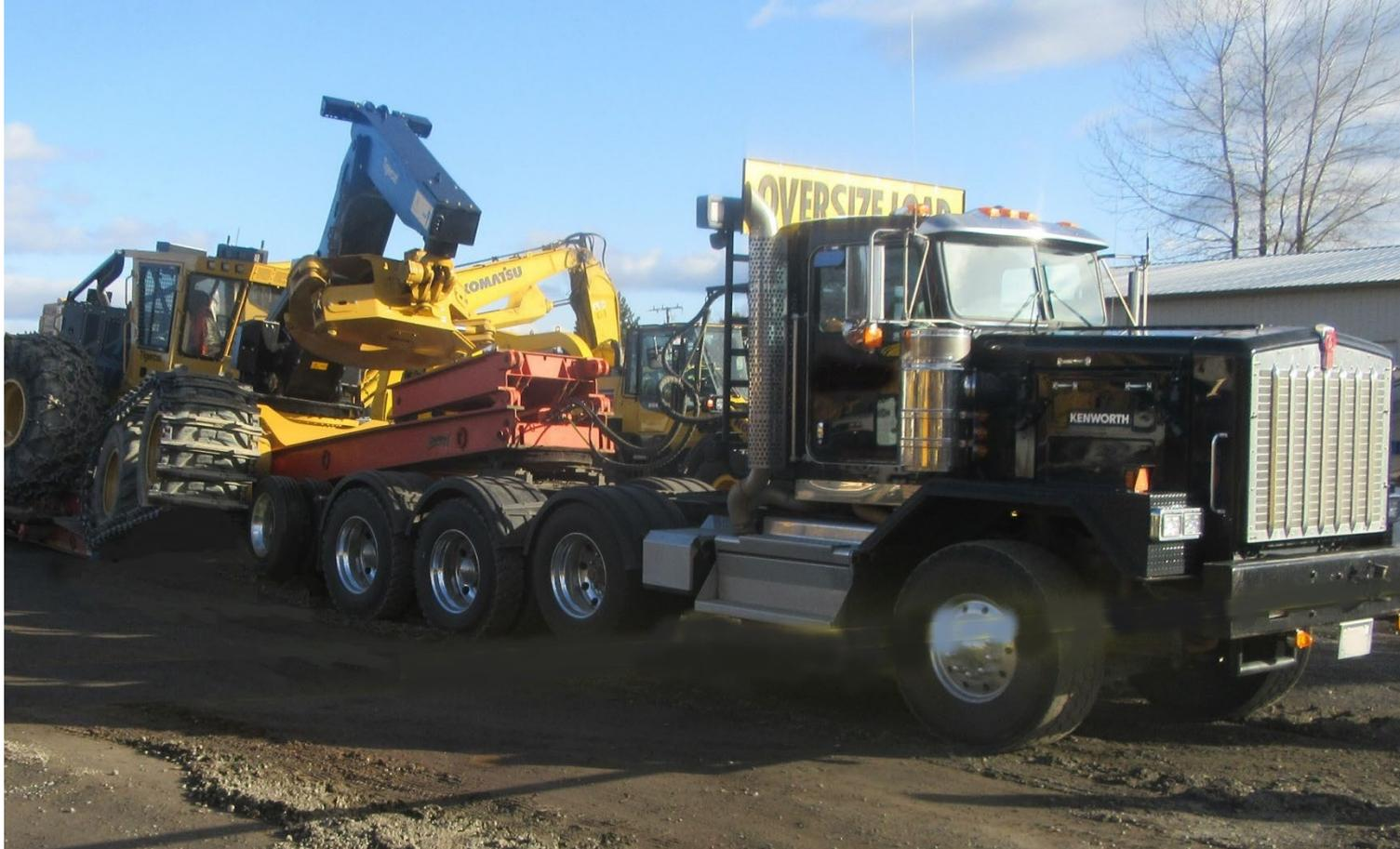
**Photo 1.** Semi-truck with skidder on detachable lowboy flatbed trailer in rear.
