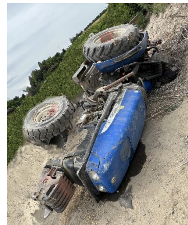
Tractor with ROPS folded down at rollover scene.
